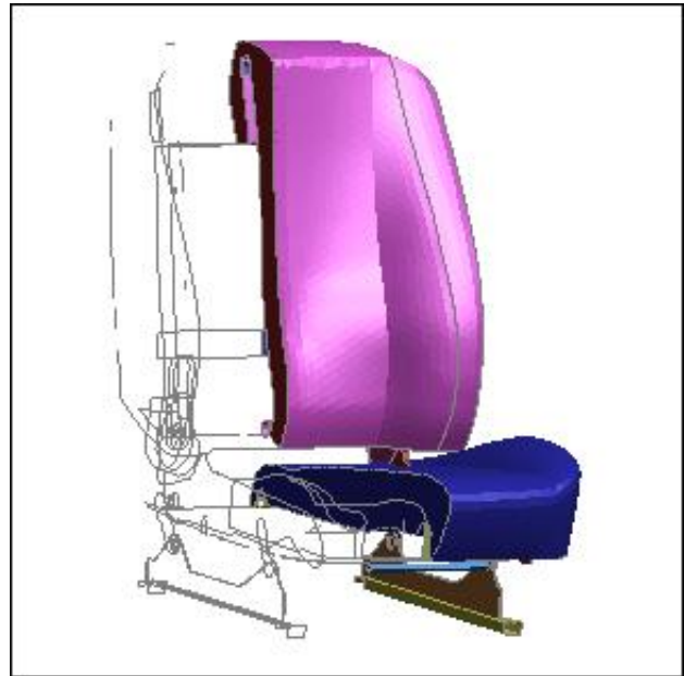
In this image the a cut section has been turned on, located roughly half-way across the seat. The +ve side (on the right) is drawn normally, the -ve side (on the left) is drawn in outline.
