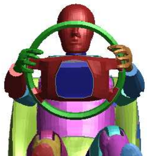
In this image the target point is the same, but the perspective distance has been increased by a factor of three, effectively moving the eye point backwards out of the paper.
